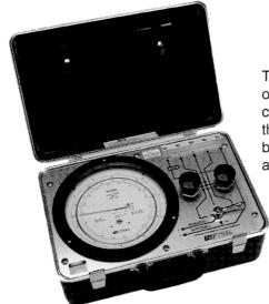
The Series 65-120 Pneumatic Calibrator provides high-degree accuracy for on-site testing and calibration service. This versatile portable test stand combines precision measurement and durable construction in a compact unit that is capable of simulating, applying, holding, regulating and measuring both pressure and vacuum. The dial, all pressure connections, and the controls are panel-mounted for easy access.
